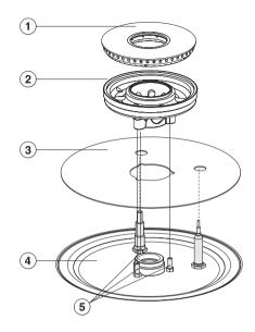
■ Place cover plate ③ over burner base ④ so that the ignitor and the ignition safety control extend through their respective holes in the cover plate. The cover plate must sit evenly over the burner base.
